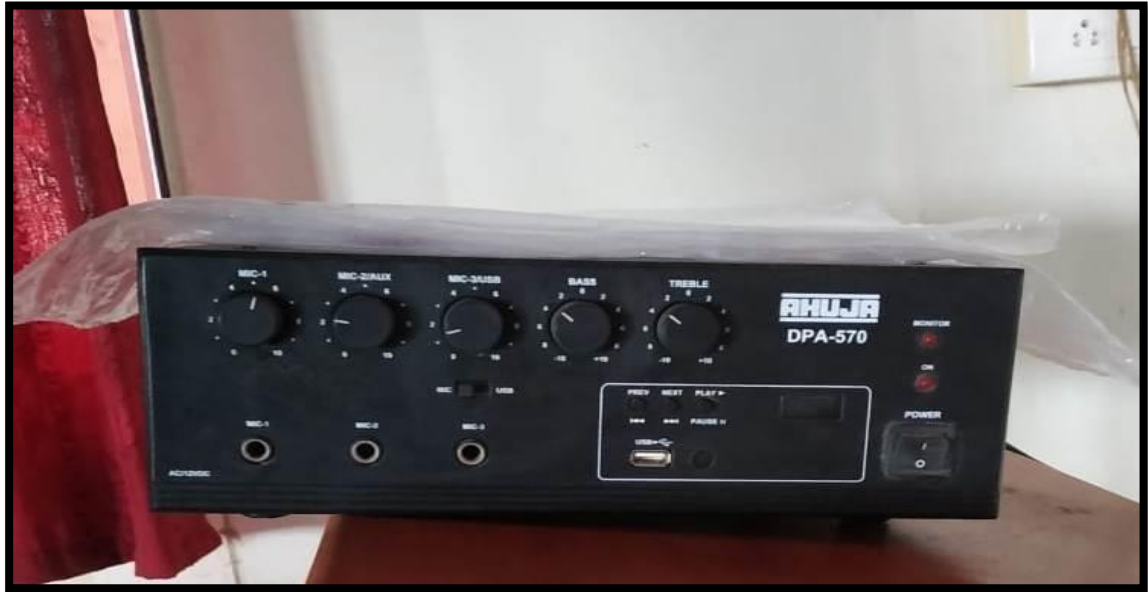
Amplifier, 50 Watts with Built-In Digital Player.
